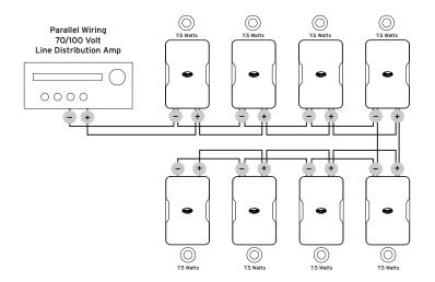
Choose a 70/100 Volt Line Distribution Amplifier based on total wattage needed to power amount of speakers at selected tap settings PLUS, we recommend, 50% additional power to cover additional dynamic headroom/future expansion. Wire all speakers in parallel.
