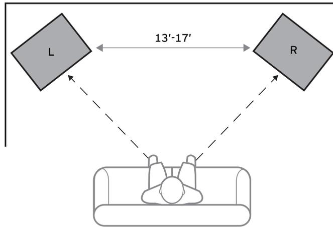
The Klipsch La Scala features a self-contained, front-firing, folded bass horn to permit placement out of the corner if required. However, because this model has less bass extension than the Klipschorn, the low frequency acoustic reinforcement of corner placement is optimal. The La Scala also offers full flexibility with regard to the amount of toe-in for the desired stereo image. Deep bass performance may also be augmented with a high performance Klipsch subwoofer.
